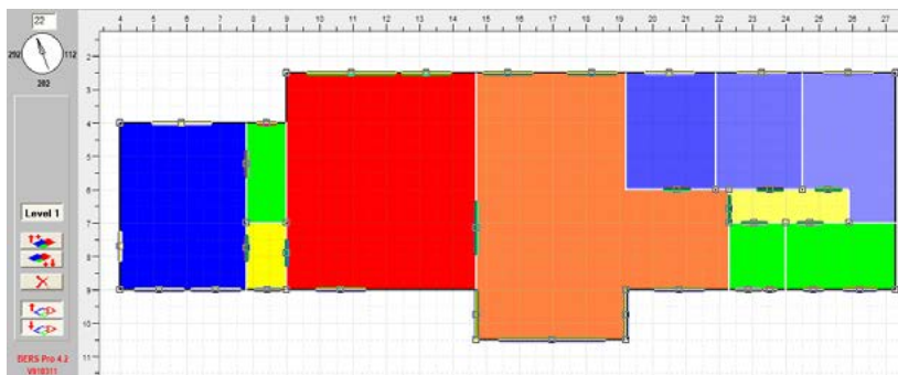
Modelled in BERS4.2 thermal simulation software Orange: kitchen/dining/living; red: living; blue/purple: bedrooms; green: laundry/bathroom; yellow: corridor
