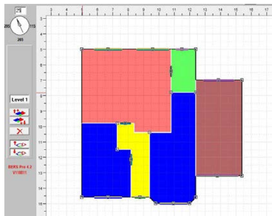
Modelled in BERS4.2 thermal simulation software Pink: kitchen/dining/living; brown: garage; blue: bedrooms; green: laundry/bathroom; yellow: corridor
