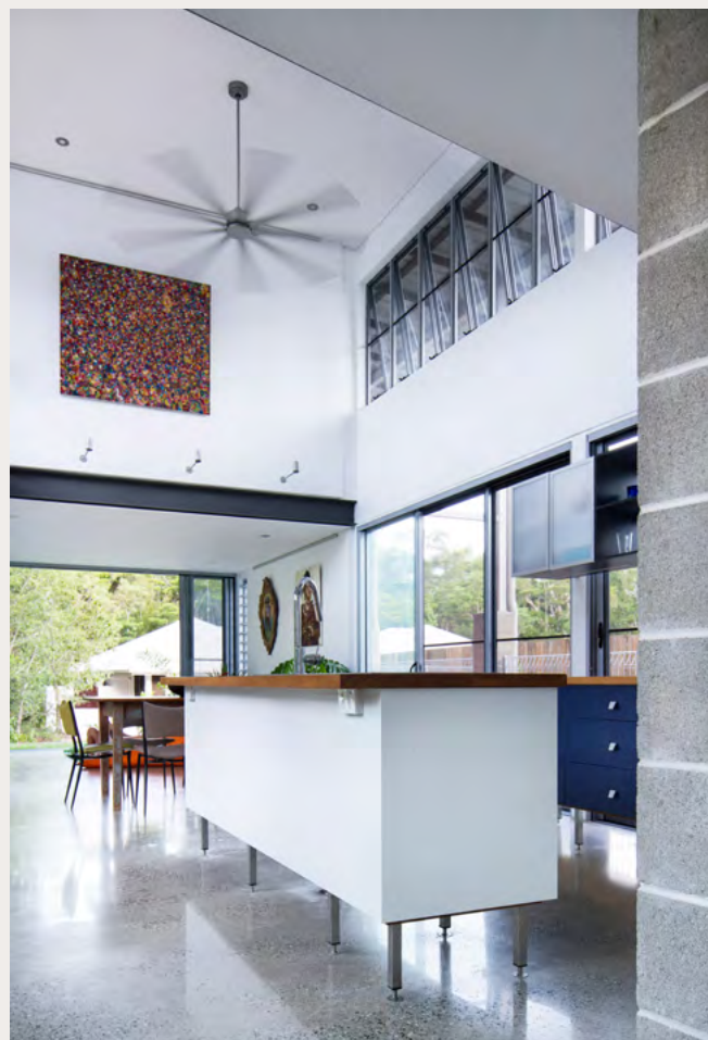
↑ The Big Small House in Cairns, by People Oriented Design, is designed to function in the tropics without air conditioning (read more in Sanctuary 38 ). Instead, the two-storey space uses cross ventilation from the sliding glass doors surrounding the kitchen and living space and stack venting of hot air to keep cool. The fan pictured is an Airfusion Resort 203cm DC model with brushed aluminium blades. Image: Nic Granleese
